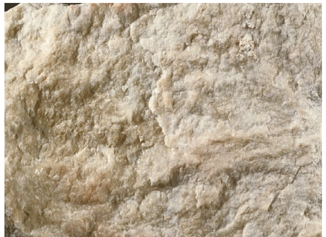
(F) Gypsum precipitates as shallow bodies of water evaporate.
